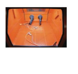
• Latex gloves and blasting guns mounted on both sides for blasting bulky workpieces from both sides without turning
