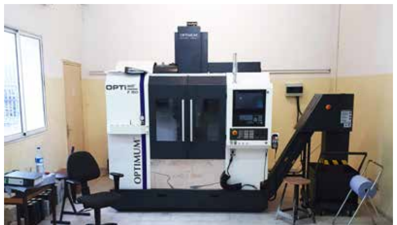
Three-axis OPTIMUM PREMIUM F150 HSC milling machine
