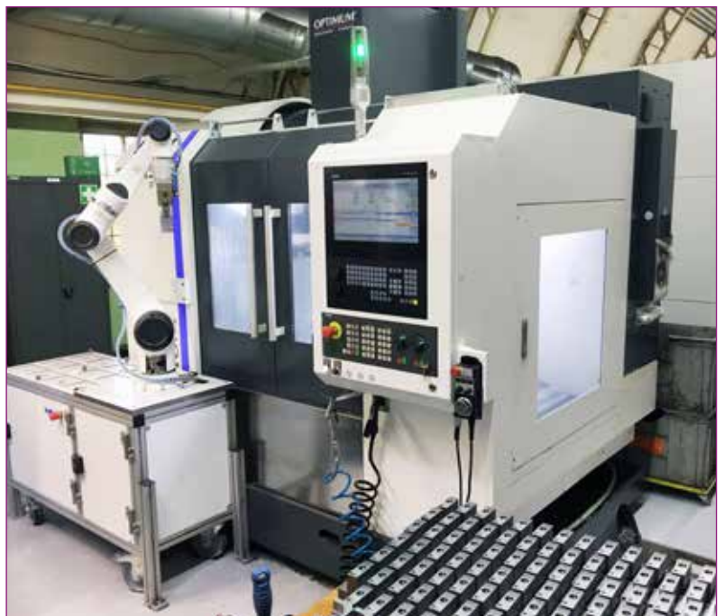
OPTIMUM CNC machines coupled to robots
