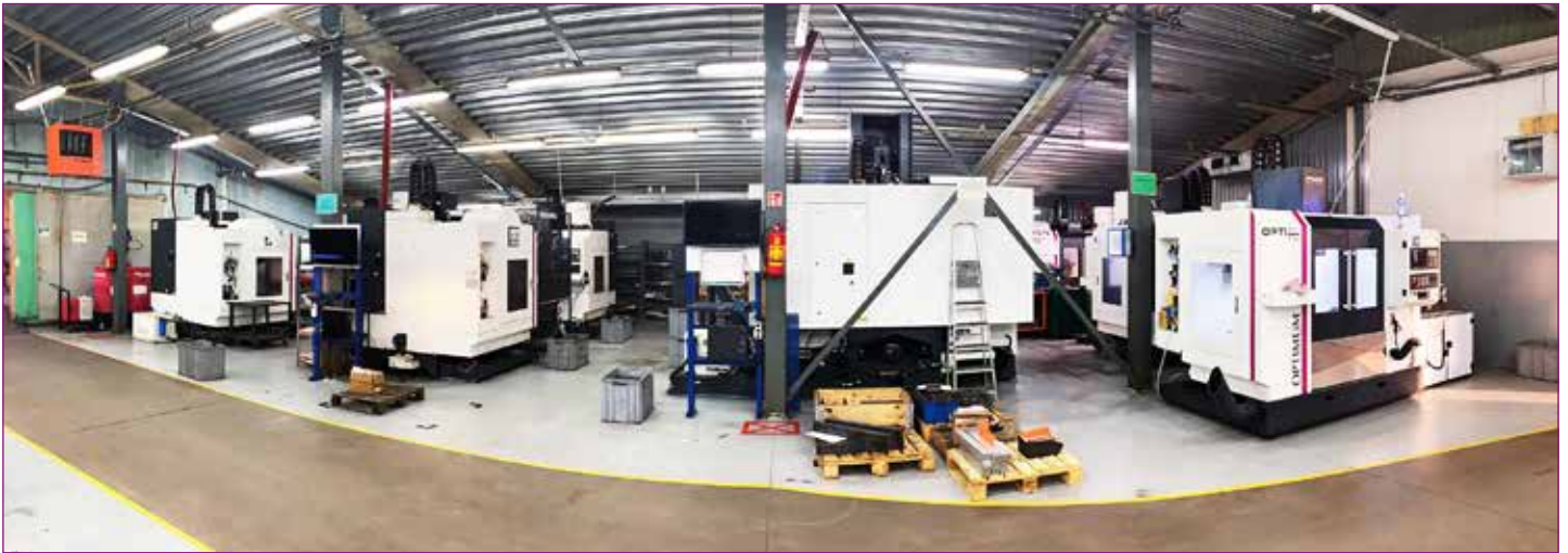
Seven F150 CNC milling machines and two F310 HSC CNC milling machines in one of Baltec's production shops
