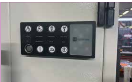
Maintenance system for monitoring machine utilisation
