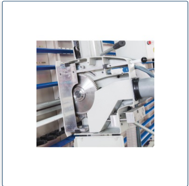
Large opening for saw blade change
