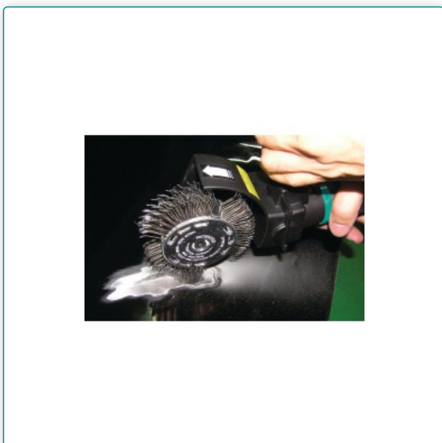
UE PRO, illustration shows carrier wheel 23 mm with rubber disc ocher installed
