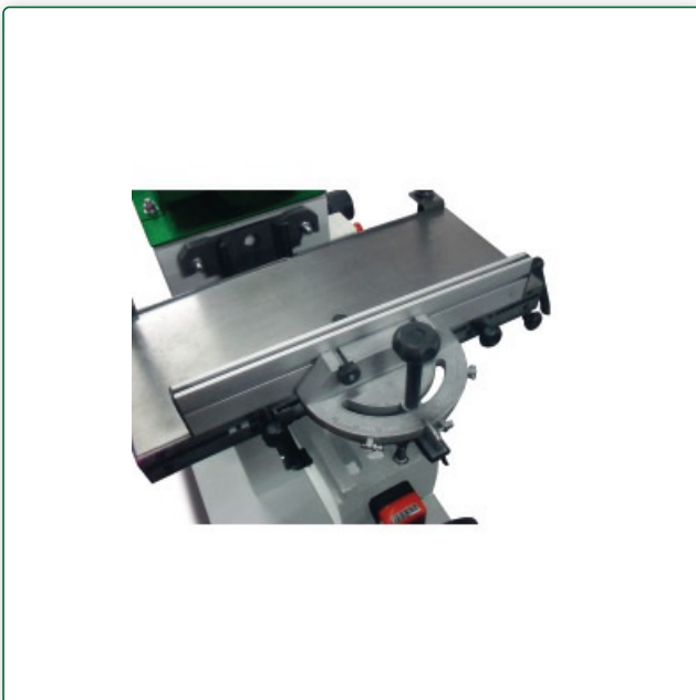
Angle stop adjustable on both sides by 60°
