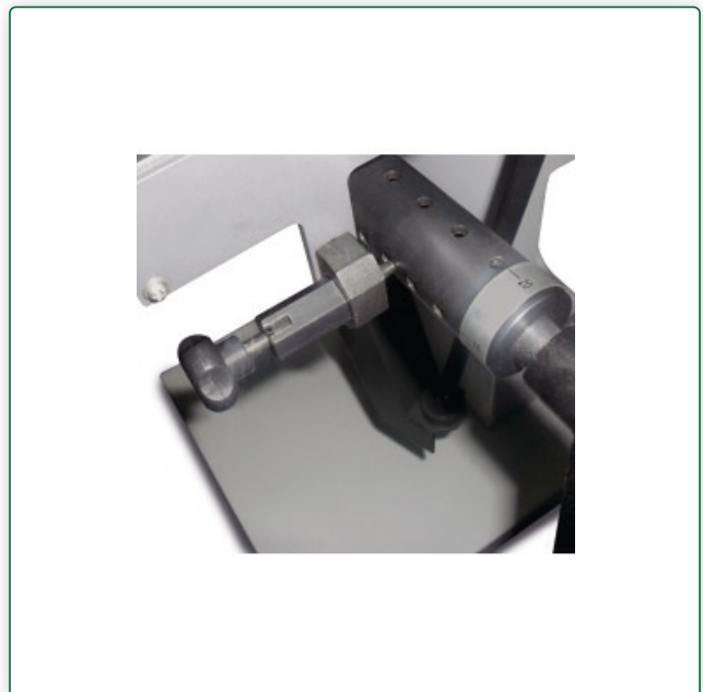
Series drilling through dowels drilling device with ratchet pitch 16/22/25/32 mm possible
