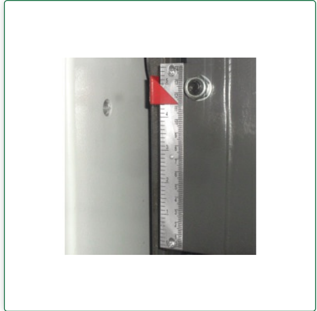
Adjusted height of workbench additionally readable on scale
