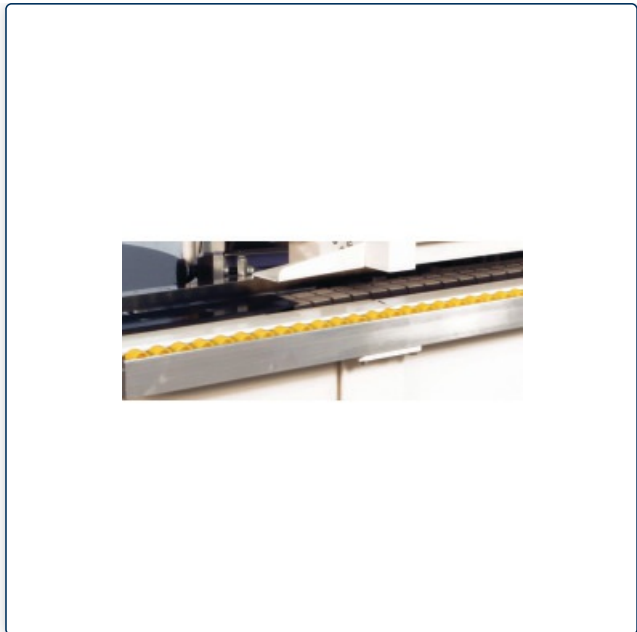
Plate transport by feed chain
