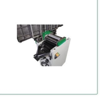
Thick table adjustment via handwheel, scale and numeric display
