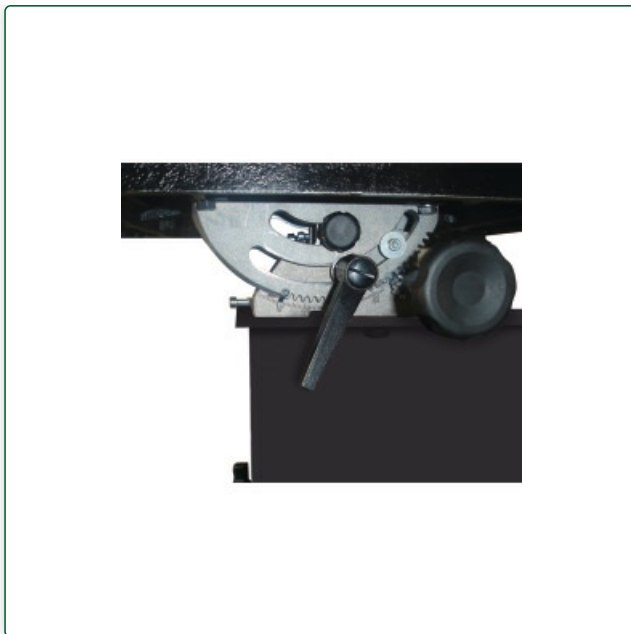
The saw table can be tilted from 0 to 45 degrees on a rocker mount
