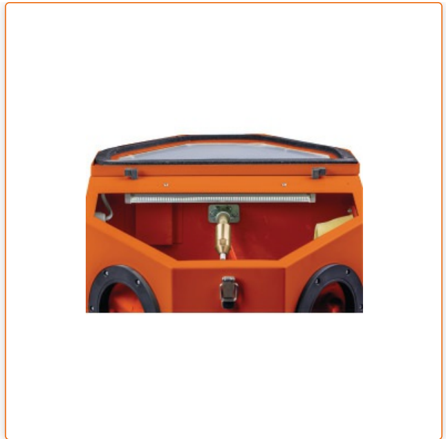
12 volt fluorescent tube with 230 volt power supply and external switch
