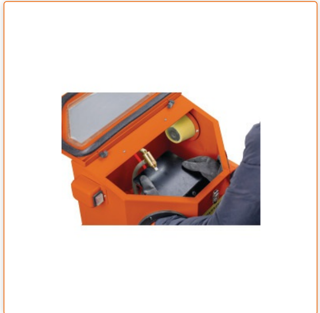
12 volt fluorescent tube with 230 volt power supply and external switch
