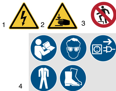
Fig. 1: Safety Labels: Warning Sign: 1 Dangerous Voltage | 2 Risk of hand injuries | 3 prohibition sign: Do not enter | 4 Mandatory signs: Read operating instructions, Wear eye protection, Hand protection, Safety shoes, Wear protective clothing, Disconnect power plug before work
