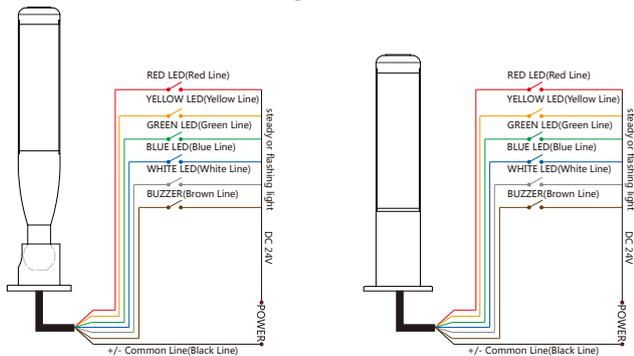
Remark: Connect the wire according to the colors if necessary.
