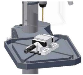
Img.4-1: seats for slot nuts
