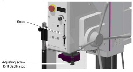
Img.4-12: Drill depth stop
