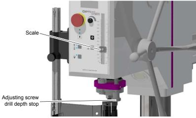
Img. 4-3: Drill depth stop
